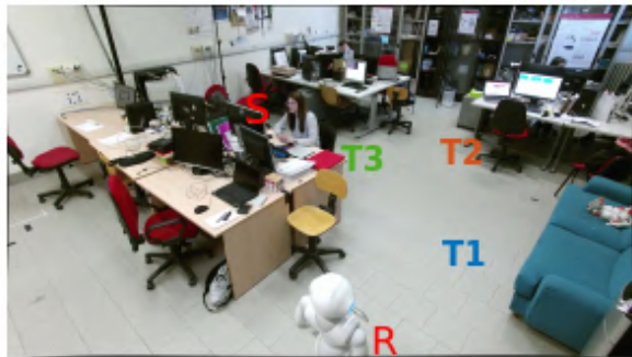
Fig. 3. The experimental environment: the user sat at position S and the robot is positioned in R at the beginning. The user was asked to mentally drive the robot from R to the three target locations T1, T2, T3 consecutively.
