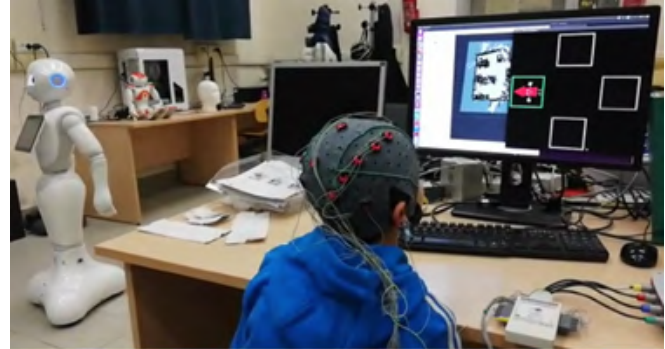
Fig. 1. A child mentally navigating a service robot by the proposed Brain-Robot Interface
