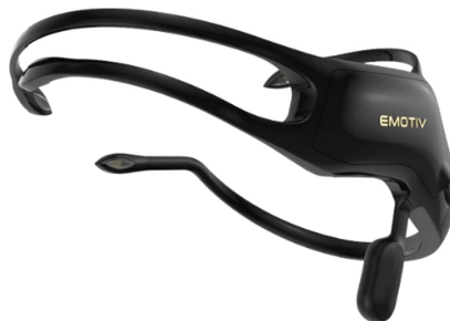
Fig. 3. The Emotiv Insight: a mobile 5 channels EEG device
