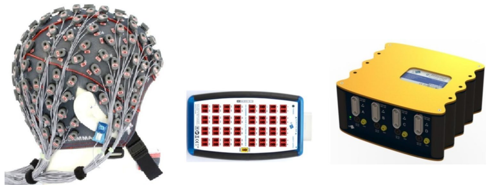
Fig. 3 g.GAMMAcap 2 with g.SCARABEO electrodes (left), driver box (middle), and g.HIamp (right) [19]
