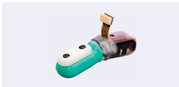
FIGURE 3. A BioTac sensor by Syn Touch. The BioTac sensor is able to perceive force, vibration, and temperatures and act as a haptic extension of a damaged or nonexistent limb. (Photo courtesy of the inventors and manufacturers of the technology at SynTouch.)
